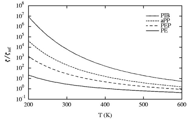
FIG. 4. Calculated friction coefficients  $\zeta/\zeta_{\text{ref}}$ , as a function of temperature at constant pressure  $p = 0.1$  MPa for the polyolefins considered in this work. The reference value is obtained for the linear chain (PE) at 413.15 K and 0.1 MPa.
