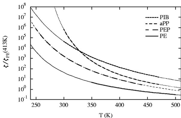
FIG. 6. Temperature dependence of the friction coefficients  $\zeta(T)/\zeta_{PE}(413\text{ K})$  extracted from experimental data. The heavy lines in the graph indicate the temperature range over which experiments were performed. cf. Table II.
