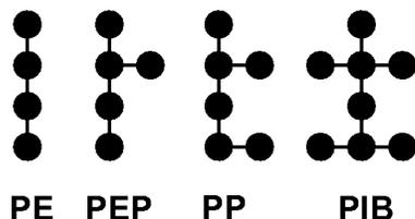
FIG. 1. United atom representation of the polyolefins considered in this work. Shown are the repeat units with four carbon atoms in the backbone for polyethylene (PE), an alternating copolymer of polyethylene and polypropylene (PEP), polypropylene (PP), and polyisobutylene (PIB).
