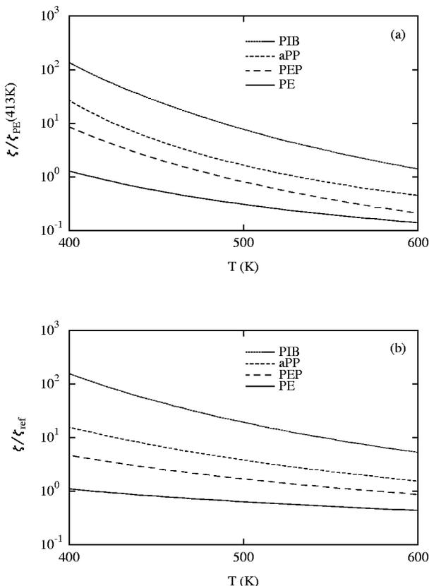
FIG. 7. Friction coefficients extracted from experimental data (a) and predicted from our simulation procedure (b) as a function of temperature at atmospheric pressure.
