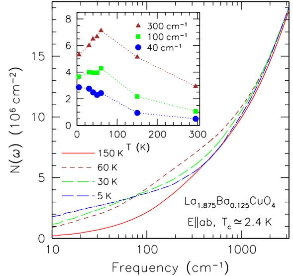
FIG. 3 (color online). The  $ab$ -plane spectral weight  $N(\omega)$  of  $\text{La}_{1.875}\text{Ba}_{0.125}\text{CuO}_4$  for several different temperatures above and below 60 K. To simplify the units, the conductivity has been expressed in  $\text{cm}^{-1}$ . Inset: The temperature dependence of the spectral weight for cutoff frequencies  $\omega_c = 40, 100,$  and  $300 \text{ cm}^{-1}$ .
